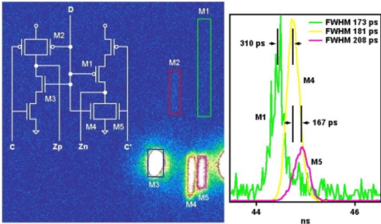
**Figure 2.** This dissection of a small portion of the image from Figure 1a shows the luminescence from the components of the tri-state driver for the D0 bond pad. The plot compares the waveforms for the visible NOR FETs.
