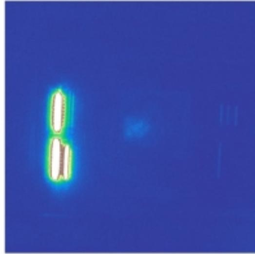
**Figure 1b.** The MX27C521pc-12 DEI from the region about the D0 bond pad with very bright nFET luminescence on the left, the bond wire imaged in reflected luminescence from the nFET in the centre and luminescence from the pFET faintly visible on the right.
