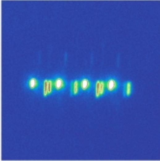
**Figure 1a.** The MX27C521pc-12 DEI from the tri-state drivers of the D0 to D3 bond pads. The four drivers are side by side. Each driver consists of a NAND gate on the left and a NOR gate on the right. The nFETs of these gates are below centre, the pFETs the faint luminescences above.
