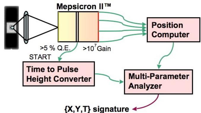
Figure 1: The DEI measurement system.
