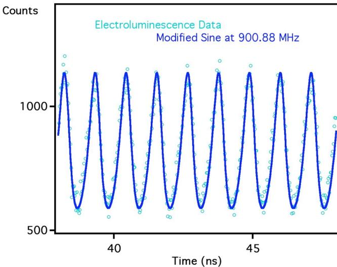
Figure 3: The LED electroluminescence data of Figure 2 fitted with the modified sinusoid as discussed in the text.
