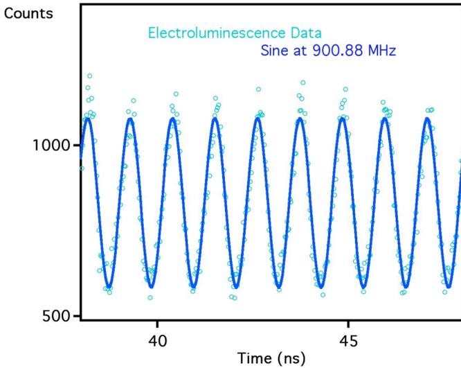
Figure 2: Electroluminescence data detected from the red LED driven at 900 MHz. The figure shows the measured data as dots, and the fit with a 900.88 MHz sine wave shown as a solid line.
