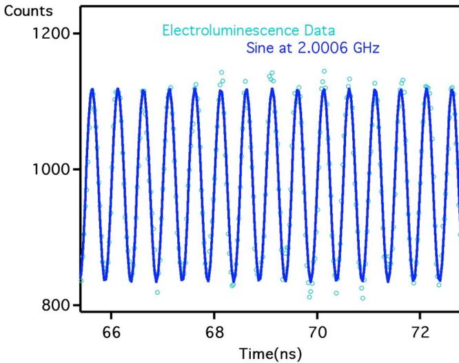
Figure 5: The AlGaAs/GaAs HBT being driven at 2.00 GHz. The figure shows the measured data as dots and the fit with a 2.0006 GHz sine wave shown as a solid line.
