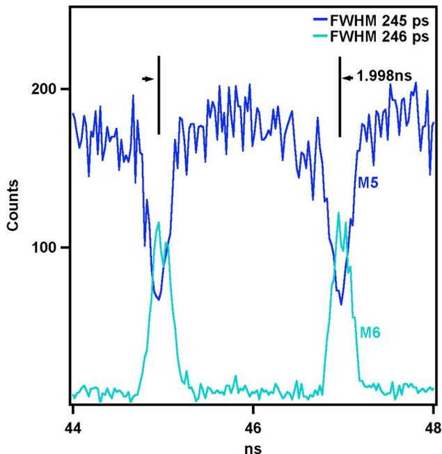
Figure 9: The luminescence waveforms from HBT M5 and M6 of the output differential gain stage.
