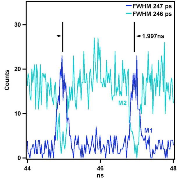
Figure 7: The electroluminescence waveforms from HBT M1 and M2 of the input differential gain stage.
