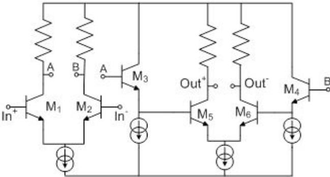
Figure 6: Simplified schematic of the high power RF differential distributed amplifier.
