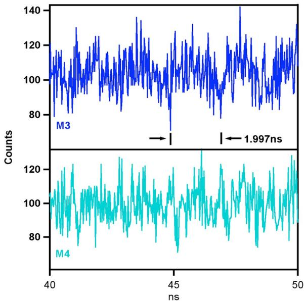
Figure 8: The electroluminescence waveforms from HBT M3 and M4 of the emitter follower buffer stage.
