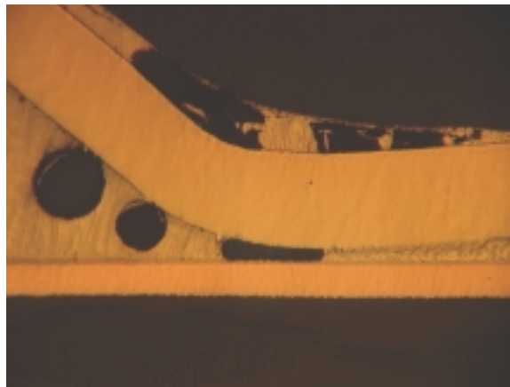
Figure 6 – Solder joint on gull wing component showing poor wetting, undetectable at visual inspection.
