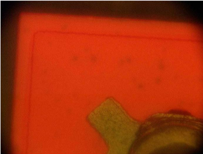
**Figure 14: Plan view emission image reveals dark spot defects and complex fabrication.**
