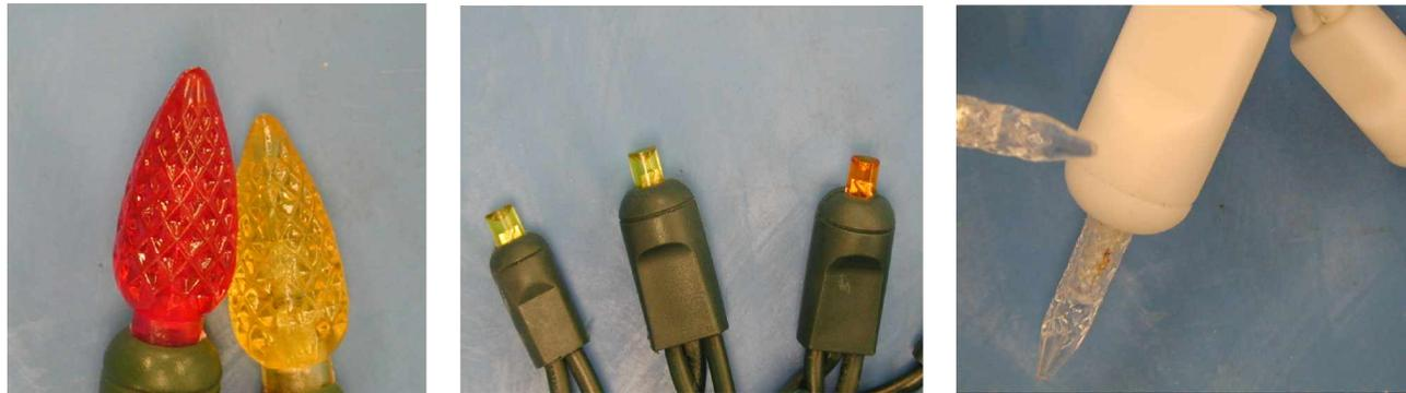
**Figure 1: Faceted, omnidirectional, and “icicle light” LED units.**
