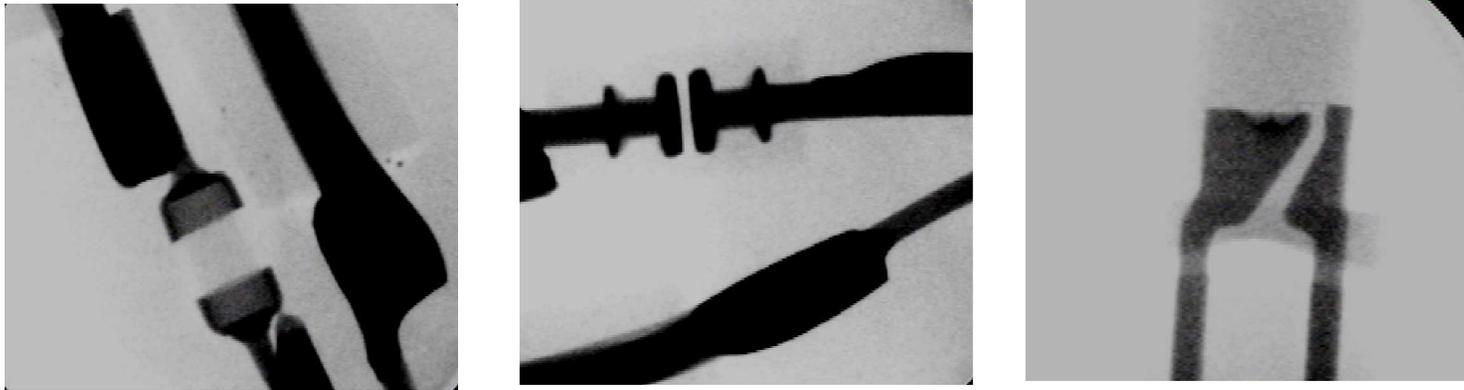
**Figure 4: X-Ray images of a resistor (left) and a diode (centre) wired in series at ends, and a typical LED (right).**
