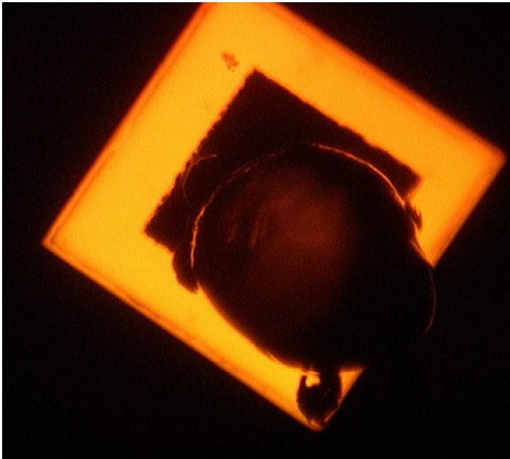
**Figure 16: Emission image of the orange LED. There is a scribe lane visible.**
