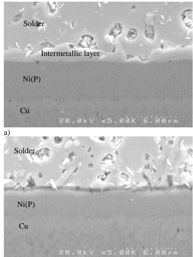
**Figure 7.** SEM cross-section images of a) a good board and b) a board affected by blackpad. On the bad board, the intermetallic layer is not continuous and the mud crack affected  $\text{Ni}_3\text{P}$  layer has formed on top of the nickel.
