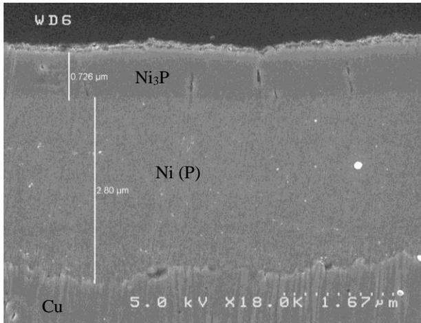
**Figure 2.** Cross-section of solder pad affected with blackpad. The Ni<sub>3</sub>P layer is less than a micrometre thick and shows cracks.
