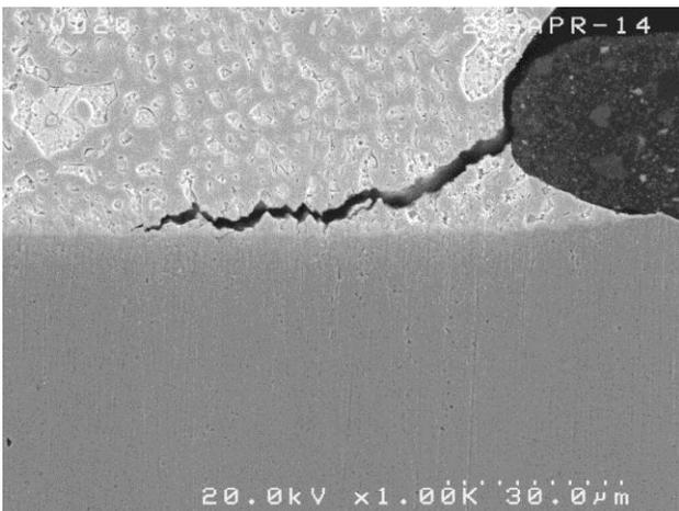
**Figure 9.** Example of a flexion crack in a BGA ball.
