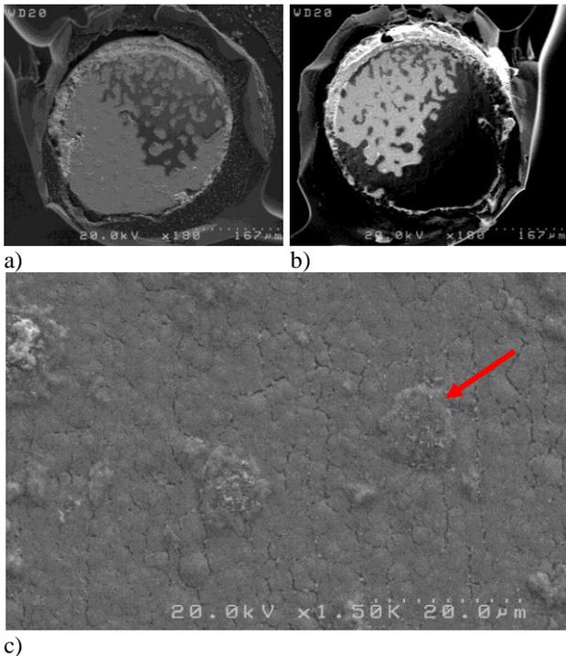
**Figure 6.** a) SEM image of a board pad after Dye and Pry test. Approximately half of the pad is covered with dye (darker region). The rest of the dye adhered to the solder ball during the pry. b) SEM image of the partially dyed
