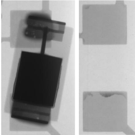
**Figure 5.** Left: X-Ray image showing poor solder wetting of a tantalum capacitor. Right: area where the capacitor has fallen. Most of the area of the pads is clear of solder.
