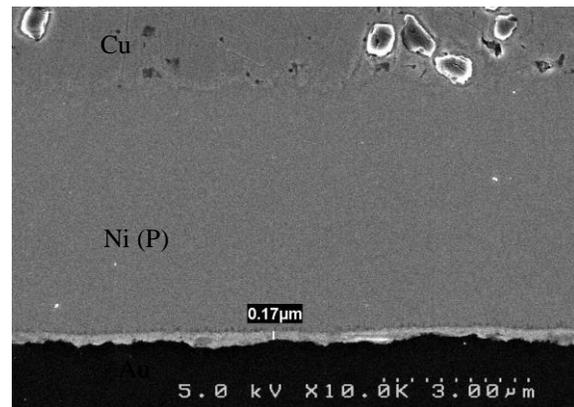
**Figure 4.** SEM cross-section image of a board affected by blackpad. A string of mud cracks is visible at the interface between the gold layer and the nickel. They have the appearance of little black dots at this magnification.
